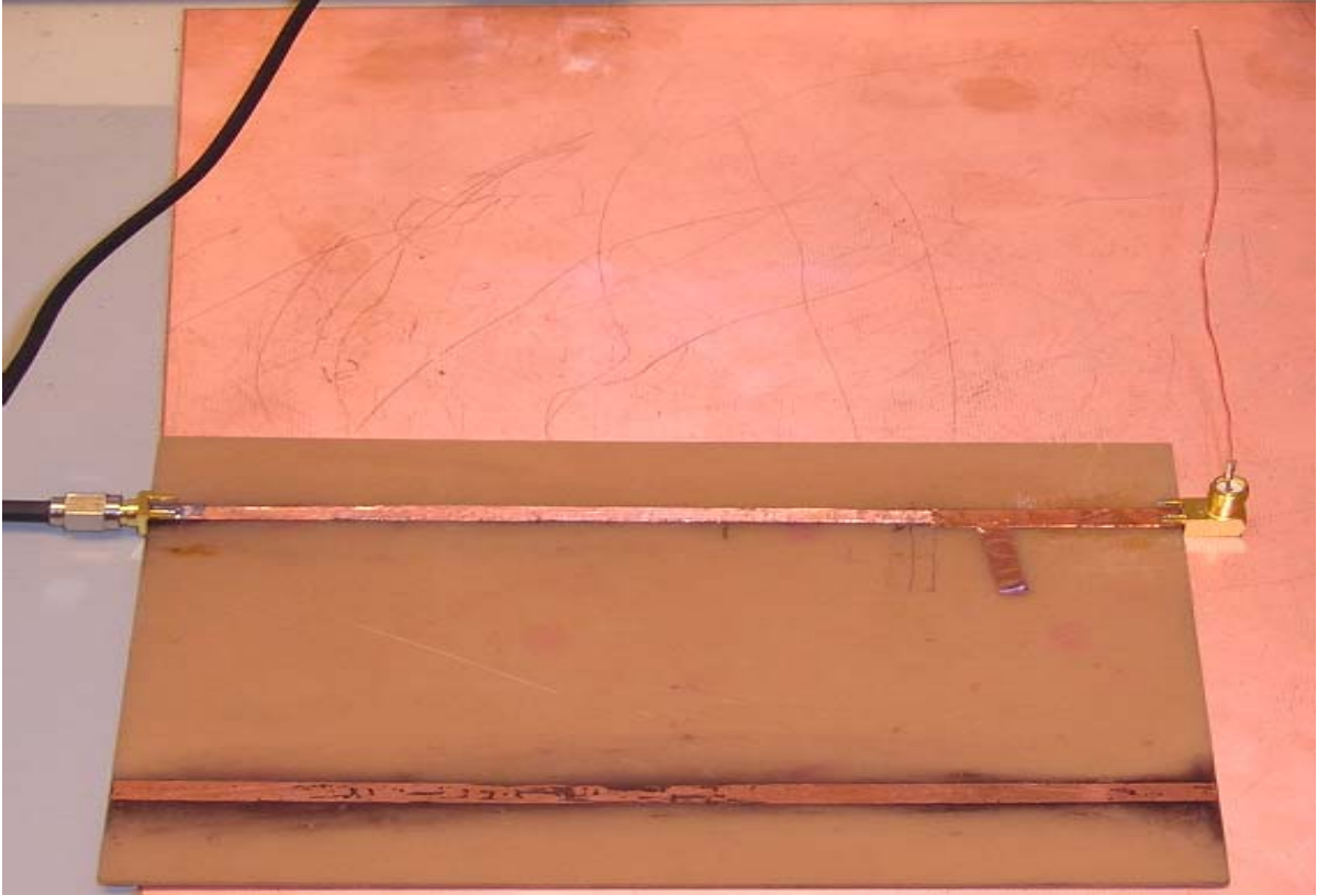
Figure 4. Monopole connected to microstrip line with open stub matching network. The antenna is made by pressing a piece of copper wire into the center hole in the connector. Be SURE to remove any varnish on the wire with sandpaper. If you are using “magnet wire”, it may appear to be a clean copper wire, but it actually has copper colored varnish on it. The open circuited PARALLEL stub is created using copper tape.
